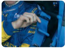
• 3" lap and shoulder straps, 4 fastening points and centre fixing with professional buckle. They are adjustable on the shoulder straps with a practical adjuster. Aircraft quick release buckle.
